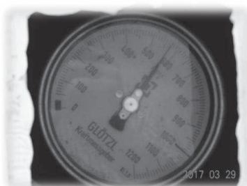
Anchored retaining beam and anchor pressure gauge.
