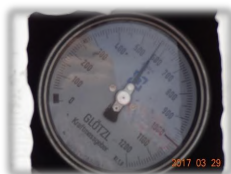
Anchored retaining beam and anchor pressure gauge.
