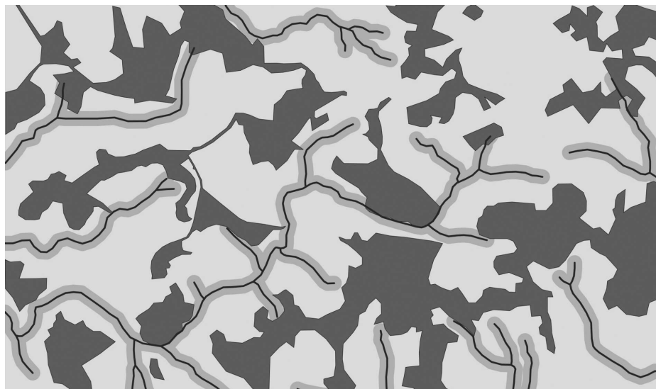
Figure 4 - Mapping obtained from the image showed in Figure 4, that in: dark brown = remnants forest; light background = pastoral and agricultural uses; dark lines = watercourses; and light brown = projection of areas of permanent preservation in order to form a strip of riparian forest with the width stated in the environmental legislation
